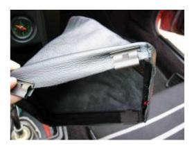
**5.** This depicts the four clips attached to the boot and frame. Note again that the larger side of the clip is on the inside of the plastic frame.
