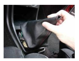
**8.** Attach/screw the shift knob back on the shift lever.
