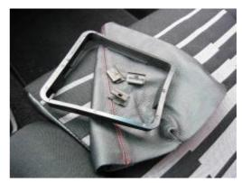
**3.** Fit the boot frame inside the bottom of the boot.
