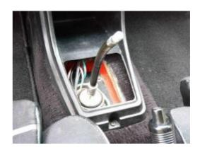
**2.** This pix depicts the new boot, original boot frame that fits in the bottom of the boot, and the original clips for connecting the bottom of the boot to the frame.
