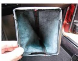
**7.** Slip the boot with the frame over the shift lever; larger side of the bottom of the boot/frame to the front of the car/console.
