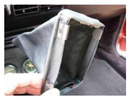
**6.** This pix depicts how the underside of the boot and frame should look. Note one side is wider than the other. This side is to be placed towards the front of the car.
