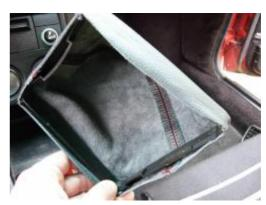
**4.** Use the clips to attach the bottom of the boot to the frame. Attach the larger side of clip to the inside of the frame.
