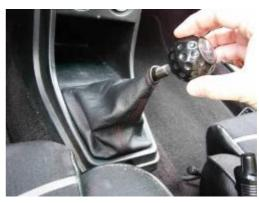
**9.** To install the ebrake boot, just slide it on top of the existing setup.
