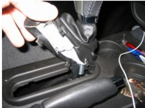
**2.** Once the shifter is removed, remove the old boot and bracket by simply pushing in the front end (the side nearest the emergency brake) until you can remove the bracket.
