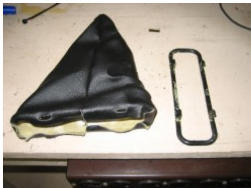
**5.** With either gorilla-glue or hot-glue, glue the new boot to the mounting frame. Remember to keep the edges flush so that the leather does not come any lower than the old rubber boot. This is extremely important.
