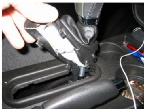
**2.** Once the shifter is removed, remove the old boot and bracket by simply pushing in the front end (the side nearest the emergency brake) until you can remove the bracket.
