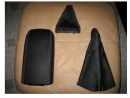
**6.** Open the center console lid and you will see (3) 7MM screw holding down the hinge. Remove the 3 screws and the lid will come right off. Under the center console lid is a plastic piece that needs to be removed to install the leather cover. There are 4 phillip screws (all the
