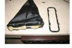
**5.** With either gorilla-glue or hot-glue, glue the new boot to the mounting frame. Remember to keep the edges flush so that the leather does not come any lower than the old rubber boot. This is extremely important.
