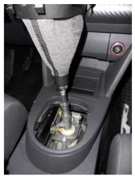
**10.** Flip the Boot to normal side and put it onto the plastic frame.
