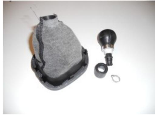
**5.** Remove the clamps from the plastic frame and remove the shift boot.
