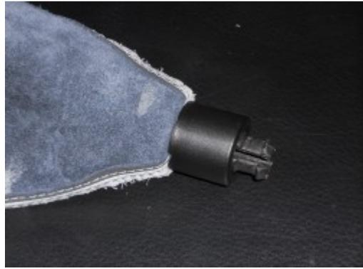
**10.** Flip the Boot to normal side and put it onto the plastic frame.
