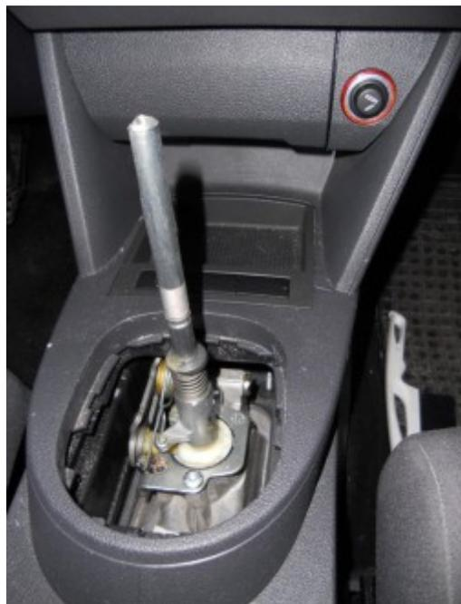
**4. With the knob off, remove the plastic retaining**
