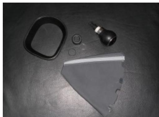
**8.** Flip the boot inside out and slide the new boot onto the knob.
