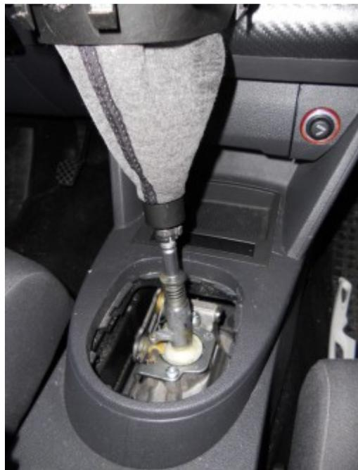
**12.** Re-install the bottom of the boot by pressing it down.
