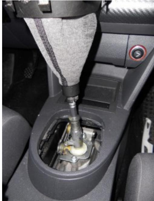
**2. Cut the metal ring around the plastic prongs holding the shift knob. Next, carefully pry the plastic prongs up while at the same time pulling up on the shift knob. The knob will then slide up off of the shift lever.**
