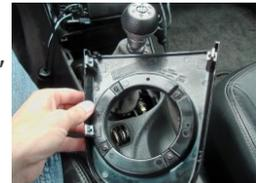
**3.** Unscrew the allen screws to separate the ring from the platform.
