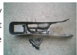
**8.** All that is left is to take out staples holding boot to boot frame (a flat head screwdriver works great). Re-staple the new boot from the bottom, then bend staple prongs over (I recommend a backboard to staple against – even into – which can then be removed so you can bend the prongs over). Alternatively, you could drill some holes through both pieces and pop-rivet them together.
