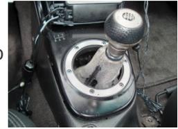
**2.** The platform around the shifter unclips. With the boot still attached, slide the platform up from around the shift rod and turn it over.
