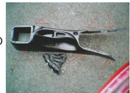
**7.** Remove the console. Slide it out of the car, make sure you do it carefully so that you don't scratch it against anything. Once out of the car, turn it over and you will see 6 screws that fasten the ebrake boot into the console bottom. Take those out then the pull boot off.
