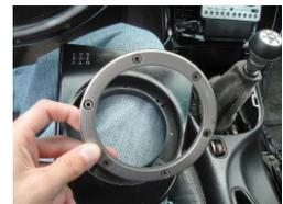
**4.** Remove the old shift boot and fit the new one around the inside ring of the platform. IMPORTANT! The new boot must fit almost perfectly in order for the ring to be able to reattach. As you can see, there is absolutely no room for slack!
