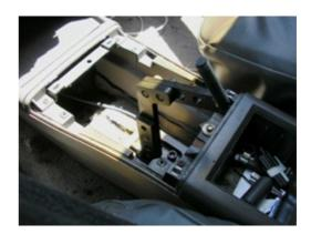
**3.** Carefully remove the metal bracket from the stock shift boot with a blade or similar tool. You may wish to clean any excess glue from the bottom of the bracket with a blade or sandpaper.
