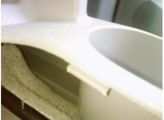
You will need to carefully snap the wire frame of the shift boot into these. There are seven altogether. (Note: The front and back only have plastic ledges that the shift boot frame butts up against. The sides actually have slots that the frame must slide into.)
