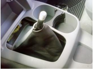
From here, all you need to do is work the frame into the plastic slots, taking your time and fitting one spot at a time. The whole boot frame will not snap into place at one time – you have to work your way around the perimeter. It is best to pinch the boot and and pull up on it since there is no good way to grab the frame.
