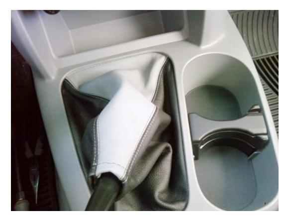
This shift boot simply snaps into place; no removal of parts is necessary. Locate the plastic slots on the underneath side of the consol.
