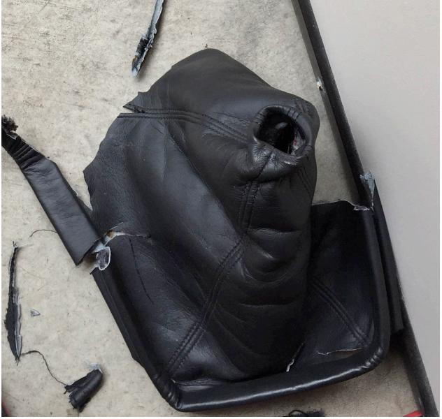
The RedlineGoods boot has a folded hem at the bottom. Wedge the wire inside the hem.
