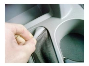
Once you have the entire frame resting in the slots, push up and back on the frame at each slot location to ensure a snug fit.
