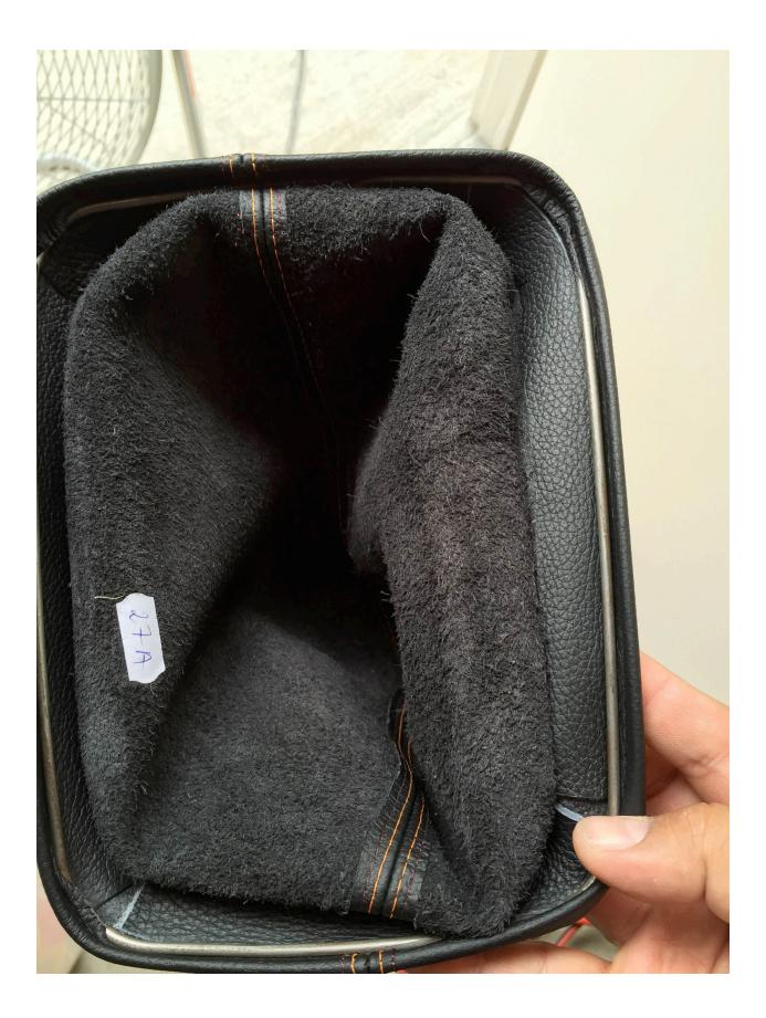
To ensure a tight fit with the consol, it is recommended that you reshape the boot frame by putting a slight arch in the wide end.
