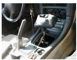
**7.** Screw the shift knob back on to the stick by turning it clockwise and pull the shift plate back down (which will pull the boot along).
