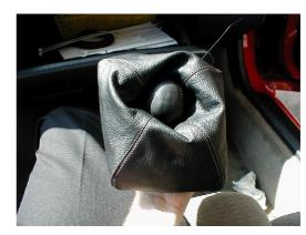
**6.** Before you install your new boot into the center console, attach the shift knob to the boot. You may use a zip-tie as shown in the picture, however We prefer rubber bands - its gives a nicer look and can always be fixed. Note: make sure the knob is facing the right way before affixing it to the boot.
