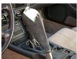
**11.** Remove the plastic zip-tie to separate the boot from the e-brake. We recommend a razor blade for this.
