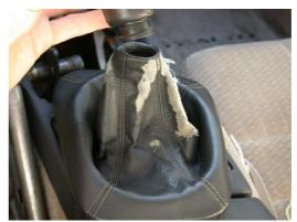
**3.** Remove the shift boot from the shift plate.
