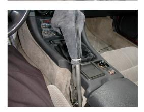
**12.** Position your new genuine leather e-brake boot into the same position and use a zip-tie or rubber band to affix the boot to the e-brake. We again recommend using a rubber band.
