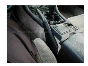
**14.** Take the boot cover that goes over the end of the handle and slide it down to expose the lower end of the handle.
