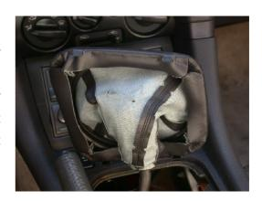
**2.** Remove the plastic zip-tie to separate the boot from the knob. We recommend a razor blade for this.
