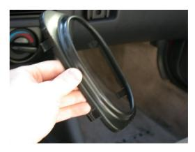
**4.** Here's were you need to be careful: Before making any slots in your new genuine leather shift boot for the shift plate hooks, place the shift plate within the boot and experiment with where you want to make the incisions. Note that the boot is customized for the 3000GT/Stealth, and as such, make sure the running edge is longer on the left than on the right. Depending on what look you
