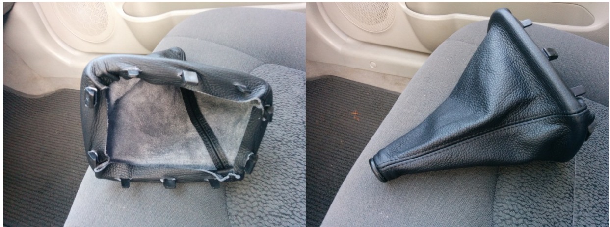
Figure 4. Shift boot placed over the plastic retaining ring and the individual attachment clips
