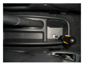
**2.** Remove the carpet liner, it just lifts up, then loosen the screw (Phillips)
