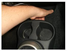
4. Pull off your stock boot, through the bottom (it is held on by a friction retainer wire, and little clips.) Remove your chrome boot top, it is held on by a slip ring.
