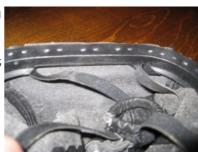
**7.** Once all the staples are removed the boot can be taken off the retainer ring.
