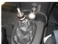
**2.** The shift boot is installed around a plastic ring that keeps the bottom in place. Gently lift up from the front of the shift boot and the ring will come up.
