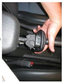
**6.** To remove the shift boot from the plastic retainer ring, you will need a pair of pliers. I found it useful to have a small metal pick or screwdriver handy as well. Carefully remove the staples from the retainer ring and take them out of the shift boot.
