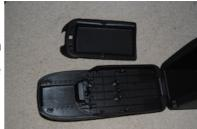
**5.** This will remove the entire lid from the assembly. Now you will see six screws on the lid. Remove these and the cover should come off.
