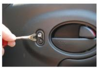
**9.** The wiring harness just unplugs from the back of the switch.
