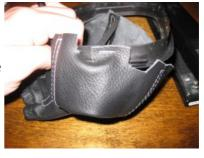
**11.** Work your way around the retainer ring by installing staples in the corners and spacing staples about every ¼ inch until you reach the opposite side of the ring. Make sure the cut sections on the shift boot fit between the plastic tabs on the retainer ring and staple once in between the tabs. Screw back on the shift knob.
