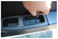
**11.** Once both are removed, pull up on the door handle pocket assembly.
