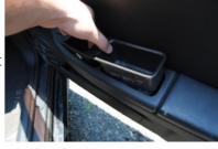
**12.** Remove the window switch wiring harness from the door handle pocket assembly. The driver's side will have an additional harness for the power mirror switch (not pictured), but is just as easy to remove.
