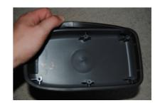
**7.** Wrap your new RedlineGoods cover around the stock cover. You can use glue to hold it down better, but I found that it was not necessary while installing mine. Now you can start reassembly. Reassembly is the opposite of removal, the only thing to note is when putting the first plastic piece back on (the one with 6 screws), you want to tuck the Arm Rest cover underneath this to hold it tightly in place. Reinstall arm rest into the car and enjoy your new leather cover!
