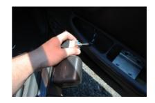
**13.** Now it's time to begin removing the door panel. In the lower corner next to the speaker, there is a screw that needs to be removed with a Philips head screwdriver.
