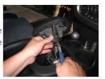
**4.** From this point the shift boot can be removed over the top of the shift lever easily and out of the vehicle.
