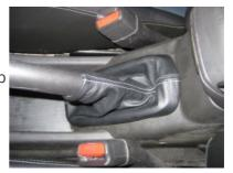
**17.** The shift boot will slide over the top of the shift lever. These have an elastic band that will stretch and there is no need for a zip tie like in the stock shift boot.
