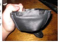
**12.** Continue attaching the shift boot around the rest of the retainer ring until you reach the starting point. Make sure your staples are fully attached and are securely holding the shift
