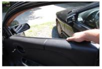
**18.** Once you have the entire panel except the top removed, pull up on the assembly (as if you were sliding it along the window) and remove it from the door.
