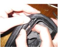
**9.** Now its time to install the boots. Let's begin with the shift boot. There are two plastic tabs on both the front and the rear of the shift boot retainer ring. The distance separating the two is not the same and the shift boot is cut differently to fit around the tabs. Match up the cuts on the shift boot with the plastic tabs on the retainer ring.
