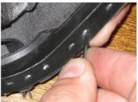
**8.** The E-brake boot is attached to the retainer ring slightly differently. The boot is pushed around the outside of the ring and is tucked back in between the outside ring and a smaller inner ring. With a bit of force, you can pull the boot of from the rings using only your fingers.
