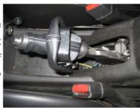
**16.** The E-brake boot will slide back over the E-brake and snap back into place on the center console.
