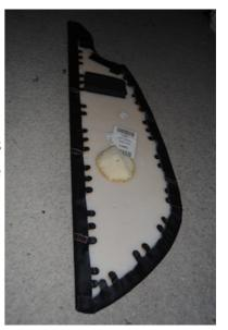
**22.** Place the door panel card back on the panel and allow the glue to dry. Gently pull up on the cards after you've let enough time for the glue to dry to make sure it bonded well enough.
