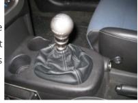
**19.** Finally, reinstall the column, spring, and shift knob. Make sure that the boot fits correctly by running through all gears before starting the vehicle. If the boot does not restrict
