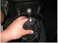
**18.** The retainer ring for the shift boot snaps back into the console just like the E-brake boot. It will be a tight fit. I suggest pulling up slightly on the boot to make sure that the retainer is fully seated.
