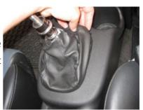
**3.** Pull the boot upwards until it is inside out. There is a zip tie used to attach the top of the shift boot to the shift lever. Locate the zip tie and snip it with a pair of wire cutters.
