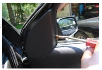
**15.** Begin removing the door panel using the pry tool. The best corner to start with would be the one where the screw was removed in step 4 (there are no push-pins in this corner to worry about).
