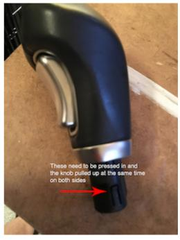
**7.** To remove shift knob from boot you will need to press into the tabs on the sides of the knob and pull.
