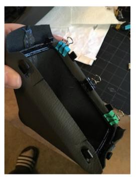
**14.** Apply glue on the inner edge and top of the frame.
