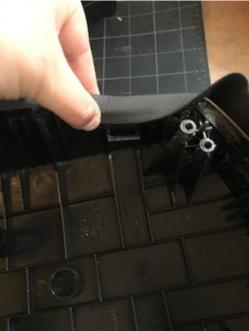
**8.** Apply vinyl cement glue on the edge and slightly over (follow old glue marks) pull leather very tight over edge and press.
