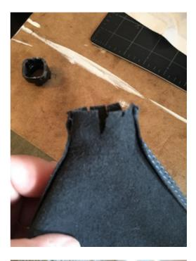
**11.** Glue sides of boot up and over black spacer slightly. using small clips, clip around top of shift boot.
