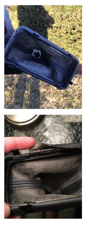
**5.** Start removing the existing leather from on the under side of the boot frame.
