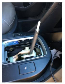
**3.** Remove the shift boot - working in sections, squeeze it around the bottom to dislodge the frame and pull off the car.
