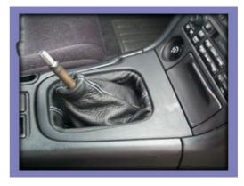
**5.** Put the trim piece back in and re-mount the shift knob and you're done with the shifter boot!
