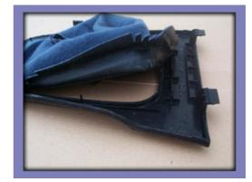
**3.** Put the new boot on the center trim piece using the poles for alignment. Put the frame back on and push the washers back on the plastic poles. Flatten the washers for better grip like in the picture.
