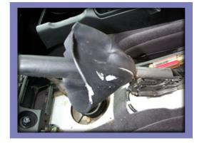
Alternatively (like on this picture) you can pull the ebrake boot OFF the handle, pull the leather onto it and slide it back on the ebrake handle.
