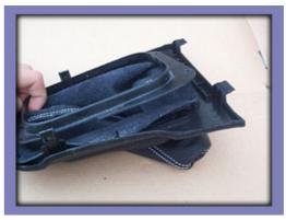
**4.** Put the top mount back on (when the boot is inside out, put the plastic ring on by pulling the leather stripes through the ring, bend the stripes around the ring and put the metal bracket back on).
