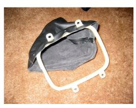
**4.** Re-mount the boot and it's plastic mount to the center piece with the 4 screws. Put the trim piece back in and re-mount the shift knob and you're done with the shifter boot!
