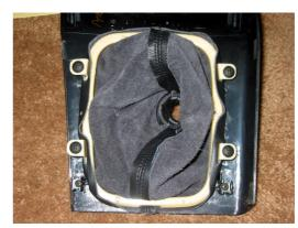
**3.** Put the new boot on the plastic mount using the slits. You do not need to heat-mount it back, it will hold up just fine without it. Put the top mount back on (when the boot is inside out, put the plastic ring on by pulling the leather stripes through the ring, bend the stripes around the ring and put the metal bracket back on).
