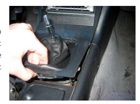
**2.** Remove the 4 screws attaching the shift boot mount to the center trim piece. Disattach the old boot from the plastic mount (just pull it off where it's heat-mounted to the plastic). Remove the top mounting (the metal bracket and the plastic ring. If you turn the old boot inside out, it's pretty obvious how to do it and it takes about 2 seconds.
