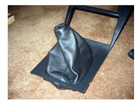
NOTE: We have changed the design of the ebrake boot to half-length. The pictures to the rigth show the old, full-length design though.
