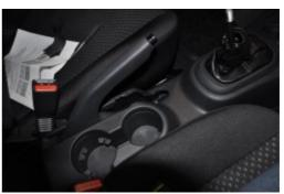
**5.** Remove the shifter boot ring from the shifter base console. !!!!!BE VERY CAREFUL NOT TO DAMAGE THE SHIFTER BOOT RING!!!!! Seperate the inner shifter boot ring from the outer shifter boot ring. Remove the stock shifter boot.
