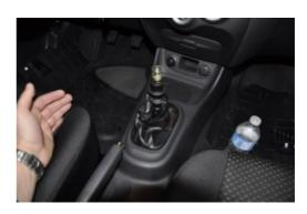
**4.** Remove the ebrake handle trim from the console using a small flat screw driver, and then remove the console from the vehicle.
