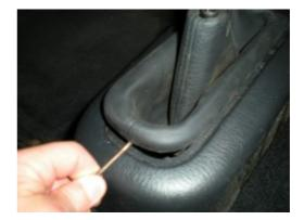
**6.** The new shift boot will need to be stretched and glued around the metal bezel and reinstalled using the opposite procedure listed above.
