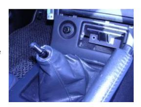
**2.** Remove the shift knob with a swift and strong counter clockwise twist. If you have never removed it before it might require significant force to loosen. Gently pull the plastic surround and remove. Remove connectors from cigarette lighter.
