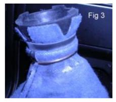
**5.** Installation of the new boot is the reverse order of the above. Replace rubber plug and metal clip then turn boot right side out. Position boot holes
