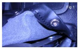
**7.** Flex metal frame and remove it from the center console. Remove the metal frame from the old boot by cutting it out.
