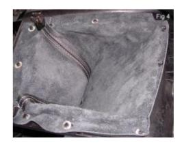
**6.** Unclip the snaps on the base of the ebrake boot.
