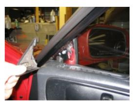
**15.** Remove the insert from the door, it's held by bent metal studs, straighten them out with a flat screwdriver.
