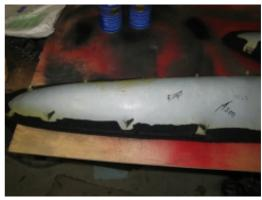
**18.** Align the leather insert with the plastic one. Start glueing from one side and keep straightening out the leather as you move towards the other side.
