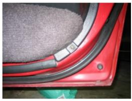
**14.** Remove the trim piece hiding the mirror, pry it off with a small flat screwdriver. Remove the door trim by pulling it up and off.
