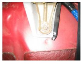
**32.** Install the rear insert over the stock one (refer to steps 21-24) and reverse steps 26-30 to reinstall the rear trim and seats.
