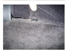
**27.** Rremove the screw by the seatbelt.
