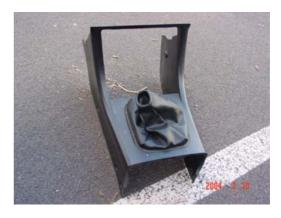
**4.** Next we want to take apart the shifter boot area. This is simply done by flipping the piece over and removing the two screws.
