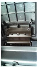
screws are exposed. These screws mount the armrest to the center console hinge.
