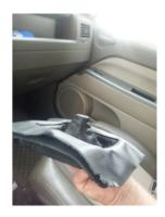
**7.** Slowly begin to put the rubber boot back onto the plastic piece, tucking the leather under the rubber as you go. It is easiest to start at one corner and work your way around.
