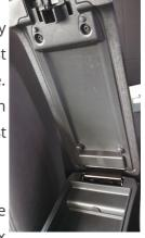
Open the armrest to reveal the torx screws on the underside. Remove the four visible Torx screws for the black plastic cover using a T20 Torx screwdriver, and place them safely off to the side.
