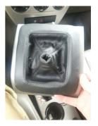
**9.** Put the boots and plastic piece back into place the same way they were removed. Slide the shift nob back on and you're done!
