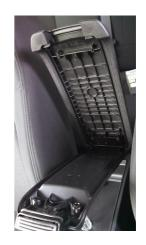
**3.** After the black plastic cover is removed, the last three remaining Torx screws are exposed. These screws mount the armrest to the center console hinge.
