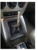
**3.** Slide the shift boot and plastic piece off of the shift lever.
