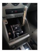
**4.** Remove the rubber shift boot from the plastic piece by flipping it over and pushing in the tabs holding them together.
