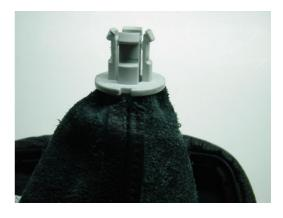
**4.** Slide the plastic retaining sleeve over the new cover and slide the shift knob back on to the shift
