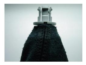
**5.** You will need to replace the metal ring, which held the knob in place. An easy replacement is a 1/4 - 5/8 in. hose clamp. Just place the clamp around the plastic prongs and tighten. Pull the cover over the shifter frame, re-install the frame back in place and you are done.
