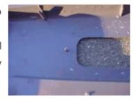
Using a sharp razor blade cut what remains of all the plastic pegs (previously securing the rubber e-brake dust shield) flush with the console top panel.
