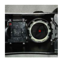
circle to release from the console. When they are free, the boot and rings can be removed from the console. It helps to have eight hands to push all the tabs at once and remove the boot. Otherwise, try to free one side and work your way around.
