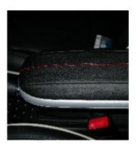
**8.** Place thumbs in middle of arm rest and 8 fingers along the top edge and gently lift up and pull towards you. There are several tabs about 3/16s tall to raise the arm rest over. There are tabs on the underside as well. (Careful, the ambient lighting wiring is behind the arm rest. Do not curl your fingers over the edge and pull out the wiring. Just keep fingers on the edge.) The arm rests are easily removed with a little nudge.
