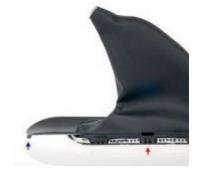
**5.** Turn the boot inside-out by pulling the base up and forward over the handle. You will find a plastic tie holding the boot to the
