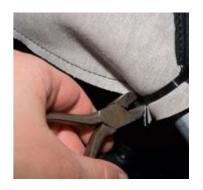
**6.** Slide the boot and handle off of the e-brake lever. The boot should still be inside-out. Extract the handle from inside the boot.
