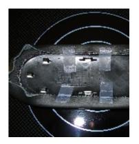
**6.** Slide the cover over the 3 front tabs ensuring the leather stays in place and then snap the rest of the tabs into place. You may have to use a flat blade to tuck leather in here and there. Once all is back together, take a razor knife and cut the tape close to the edge and remove from leather.
