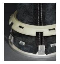
The leather already has some slits in to go over the tabs in the chrome ring. Only about half of the slots matched the tabs, so I had to enlarge some and create one or two new slits. Line up the front seam in the leather with the front marker on the chrome ring. On my boot, the two seams were not identical. Note that the boot is inside out and the rings are upside-down.
