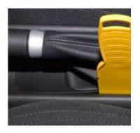
**4.** There is a tab in the front end of the boot base. So, best to tip it up from the back end and slide it back to release that tab (blue arrow below). I found it impossible not to break a couple of tabs off of the e-brake boot. These two tabs (red arrow) stick out farther than the others and are rather fragile. They don't seem critical in holding the boot in place. Mine stays down quite well without them.
