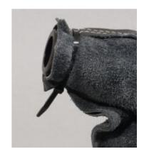
**16.** With the boot still inside out, slide the handle onto the brake lever as far as it will go. Pull the boot back far enough to see that the button is sticking all of the way out of the handle.
