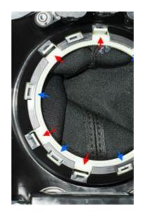
**10.** Next, try to gently release the small tabs to remove the bottom ring from the top chrome ring. The tabs are very fragile. I broke most of them and repaired them with CA glue. However, they are not really necessary as tabs, but they do help hold the boot in place while assembling.
