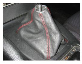
**9.** Cut off your original e-brake handle cover along the threads. Slide the Redline Goods handle down the plastic handle until it looks like this. Glue the tip down onto the plastic handle.
