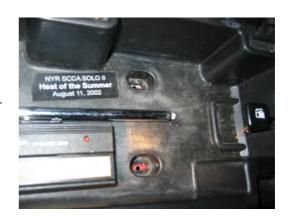
**2.** Lift out the ashtray / cupholder, and remove the single recessed screw.
