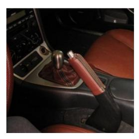
**10.** Slip fit the e-brake boot over the plastic e-brake cover. Tuck the excess leather into the slot in the carpeting.
