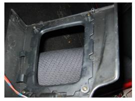
**5.** Detach the old boot, note the installation method. Also note the wiring harness needs to go under the wiring guide belt into the plastic boot holder.
