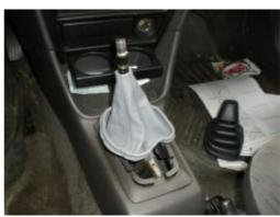
**7.** Start either at the front or back, and gently unfold the boot over the holder.
