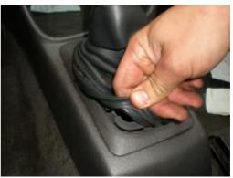
**3.** Work around the boot, gently pulling outward until the whole boot has been released from its holder.
