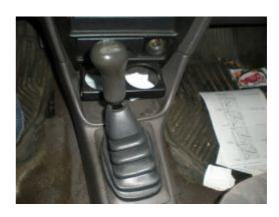
**2.** Gently pull out and up on the edge of the stock shift boot. It will release from its holder.
