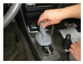
**6.** To make the install easier, fold up the bottom edge of the boot.
