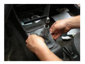
**8.** Make sure that you tuck the edge inside the holder to make sure it is secured. A flat head screwdriver used with care (so you do not damage the boot) may be useful to help you tuck the edges in.
