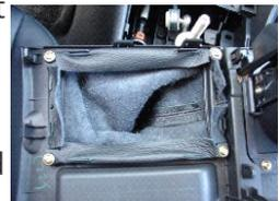
6. Once the cover is removed, flip it over. There are four Philips headed screws that need to be removed to remove the shift boot. Take these screws out, and the boot will come out (with the rectangular plastic holder).
