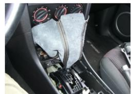
6B. Tighten zip ties and turn shift boot from inside out back to normal. It took me a while to get it just right. There isn't much room on the bottom of the boot so I didn't even bother securing it. It remains pretty snug when you place the console back together again.
