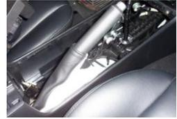
8. Simply put the new boot in place and put everything back together. You will need to remove the top trim piece from the old boot and install it on the new one as well.
