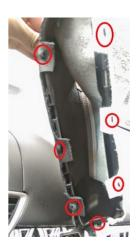
**9.** Now it is time to move on to the front trim and the shift boot. Pull upwards on the trim, while being careful not to break the clips. While the order you remove the clips doesnâ $\in$ <sup>M</sup>t particularly matter, it is easier to do it in the order as shown, RED, GREEN, then BLUE.
