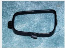
**5.** Apply adhesive to the both shift knob retainer and new shift boot and place the end of the boot inside the ring, it is easier to do this if the boot is inside out. With adhesive on both the ring and the boot pull it right side in and press together.
