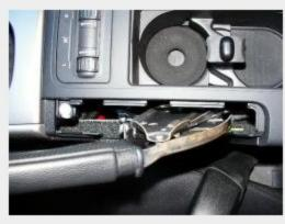
8. Remove boot from plastic retaining piece.
