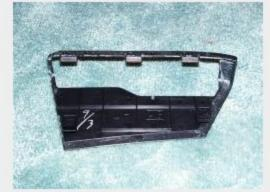
**10.** Reinstall the bezel with the new shift boot back in the center console piece. Reinstall everything else.
