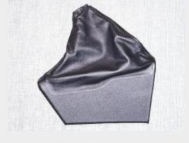
**9.** Apply adehesive to both new boot and retaining piece, fit boot around retaining piece and press together. Make sure to fit it exactly to the retaining pieces shape.
