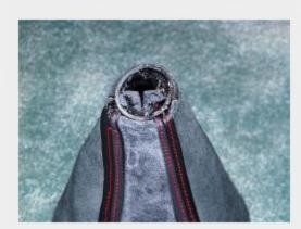
**6.** Apply adhesive to both new shift boot and plastic retainer ring and fit the boot around the retaining ring.
