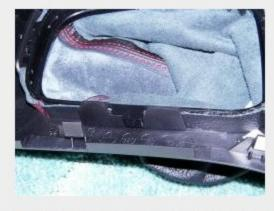
**4.** Remove the staples. Peel the old boot from the plastic bezel then pull the boot inside out and remove the shift knob retainer.
