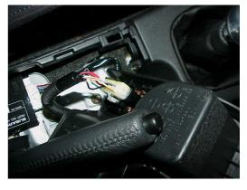
**3.** Remove the front part of the center console. Just pry gently and it should remove. Don't use excessive force, if you come across an obstruction, figure it out, don't force it out.
