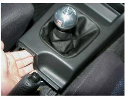
**4.** Boot is held in by a plastic frame and tiny metal rings on fragile plastic pegs. Use needle nose pliers to grab. They may bend but it's OK - they can be pounded flat with a hammer on your garage floor.
