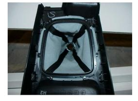
**5.** Once all the metal rings are removed, 6 of them, the boot and bracket are free. The boot is glued to the bracket. Shift knob requires very small screwdriver and a bit of prying to be freed
