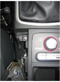
**4.** Under the Ebrake bolt is a bolt that needs to be removed (circled in red)
