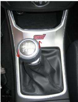
**6.** Remove the shift knob by turning it counterclockwise
