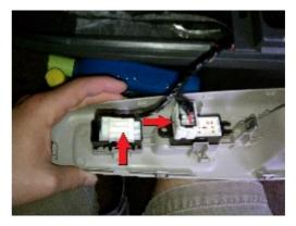
**5.** Turn the armrest over, and you'll see the plugs for the power windows and locks. You'll need to use the small flathead screwdriver to push in the tabs and remove the plugs
