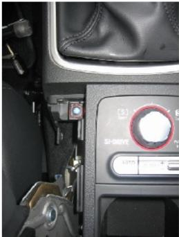
**5.** Slide the entire center console towards the rear of the car. DO NOT LIFT TOWARDS THE ROOF OF THE CAR AS YOU WILL BREAK THIS LITTLE WHITE CLIP (circled in red). When you reassemble the center console later, it helps to separate this clip into two pieces and place the upper part in the center console.
