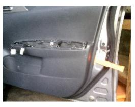
**8.** After prying the panel off, remove the door lock and door pull cables from the door panel. Remove the plastic door panel and lay it on a stable, soft surface, with the back side facing up. (Be careful not to scratch the other side - the plastic is soft and gouges easily!) Locate the 4 white plastic rivets which hold the stock vinyl armrest to the door panel). Using a drill and approx 1/4" bit, drill these rivets out. Only drill out
