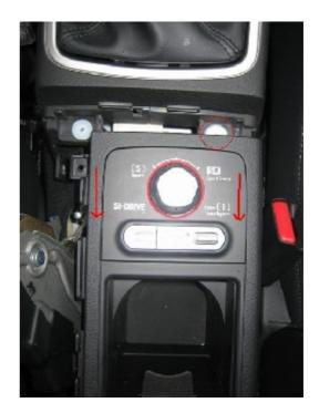
**6.** Remove the shift knob by turning it counterclockwise
