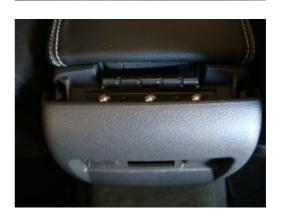
bottom cover. This is just snapped in place. Use a nylon trim removal tool or similar. You don't have to remove the large metal plate to get the cover off, you might in order to ensure you don't snag it when re-installing the cover.
