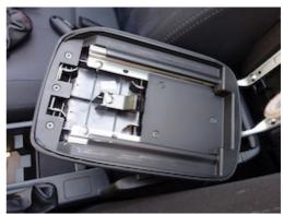
**3.** Once removed you can install the leather cover. Note the two metal bars are sharp - be careful in order not to get cut.
