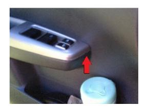
**5.** Turn the armrest over, and you'll see the plugs for the power windows and locks. You'll need to use the small flathead screwdriver to push in the tabs and remove the plugs
