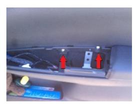
**7.** Using a panel popper or other long flat wedge, pry the door panel up from the side. Use your fingers to pry the panel off the door, popping the individual pins from the door. Short, quick jerks work best
