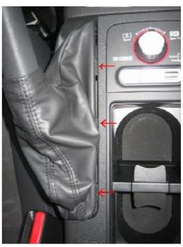
**3.** Once the tabs have released, just slide the entire boot over the handle. You will now need to remove the old boot from the plastic frame. The leather is bonded to the plastic frame with adhesive and you can use a hair dryer to soften the adhesive and gently peel off the old boot. Super glue works well to attach the new boot.
