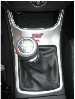
**7.** Then grab the tray and the shift boot portion and pull it straight back as well. However BE VERY CAREFUL, as there are small fingers that hold the whole assembly to the lower part of the dash.
