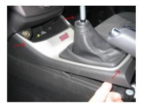
**8.** Flip that piece over (be careful not to disconnect the wires) and remove the shift boot and frame by pushing on the tabs (see red arrows)
