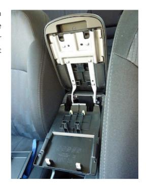
**2.** Remove the six black screws that hold the bottom plastic cover.
