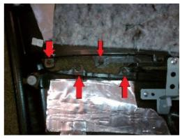
**13.** Install the newly wrapped armrest back into the door panel. Align the mounting nubs with the rivets you drilled out previously. Mount the armrest using the #12x1/2" screws. Depending on how much you drilled out, you may not need the washers. Hand tighten until the armrest is flush
