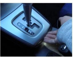
**2.** remove the lower trim piece and set it off to the side. Remove the shift knob (unscrew counterclockwise)
