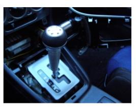
**3.** fit the shift boot, making sure to align the seams how you would like them oriented, I chose to have the seams point to the four corners of the trim piece.
