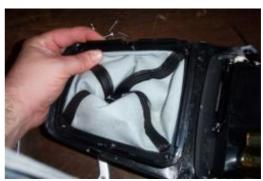
**4.** The e-brake boot is held in by one clip nearest the storage compartment. Unsnap this clip and give the boot a gentle tug and it will come out. Once again the boot is glued to the frame and needs to be pulled of.
