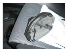
10. Once they are all off and the old boot removed from the bracket, place the new boot over the bracket and align the boot correctly with the clips. You may need to trim the boot a little to make it fit perfectly.
