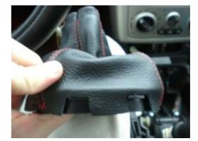
**11.** To secure the boot to the boot bracket, you can staple or replace factory staples (or zip tie/super glue) but I just sewed through the original staple holes and it worked great.
