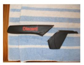
**16.** Cut the e-brake handle cover as shown and discard the front portion as it will not be needed for this installation.
