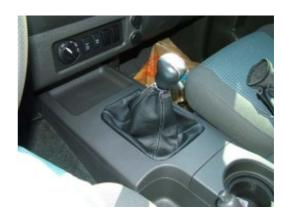
**9.** Use a flat screwdriver or a trim panel removal tool and pry one end of the boot from the center console. You will need to cut the boot from the plastic trim rings using a razor blade or utility knife. You must save the ring as the new boot will be glued back to the ring.
