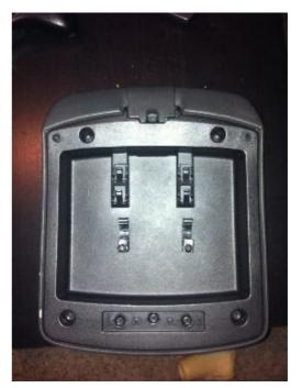
**13.** I chose to put the leather over top of the stock vinyl. It covers it up nice, and the stock vinyl provides a little extra cushioning. Fit the leather over top of the console lid and then pull it tight, and put the inner plastic piece back on top.
