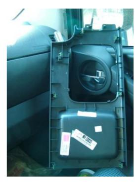
**6.** This is what the boot will look like once removed. You will need to cut the boot from the plastic trim rings using a razor blade or utility knife. You must save the ring as the new boot will be glued back to the ring.
