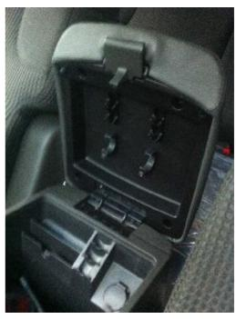
**12.** Remove the four torx screws in each corner of the inner plastic, and then separate the plastic
