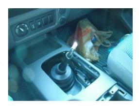
**4.** Remove the M/T finisher bezel. This is accomplished by pulling up on the retaining clips on the edge closest to the cup holder finisher and then pulling the piece towards the rear of the vehicle.
