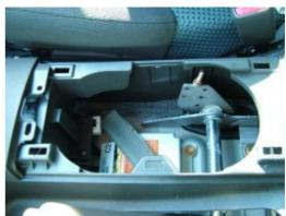
**3.** Unscrew the shift knob. In some cases, a good twist is needed. Other times, you may need to break out the locking pliers. Wrap a towel around the knob so that you don't mar the knob, lock the pliers, and twist. The boot has already been removed from the picture.
