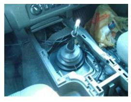
**5.** Remove the shifter boot by undoing the clips that surround the boot and attach to the M/T finisher bezel. This is what the finisher would look like with the shifter boot removed.
