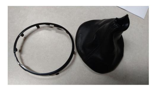
5) Line up the trim ring with the new boot. The notch cut in one side of the boot will align with the notch in the trim ring (about the 10'oclock position in stock orientation). The first picture shows the correct orientation of the trim ring when snapped into the console. Note the notch at the 11 o'clock position and the grab point you used in step 2 at the 3'oclock position.
