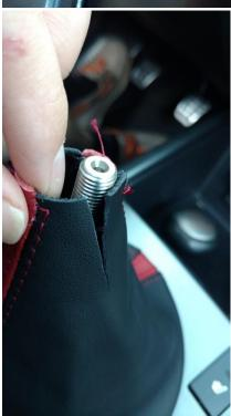
9) Once you have the boot on, flip it inside out again. Align the top (skinny) part of the boot to cover the groove on the shifter. Then zip tie the boot to the shifter. Note: if you cut a slit try to get as much of it below the groove as possible to minimize its appearance. If you have leather sewing equipment, you can also add a couple of stitches to close the cut and provide a more professional appearance.
