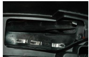
**10.** With the boot installed, replace the console in the vehicle by following the steps from removal in reverse order. Carefully work the e-brake handle through the new boot as you lower the console into position. Before you attempt to reinstall and fasteners, check to see that your seat belts are out of the way and you haven't trapped any wires under the edge of the console.
