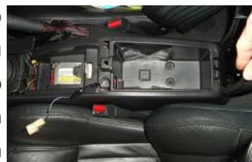
7. Turn the console over and find the e-brake boot. You'll see how it's retained upon examination. The first thing to do is remove the metal
