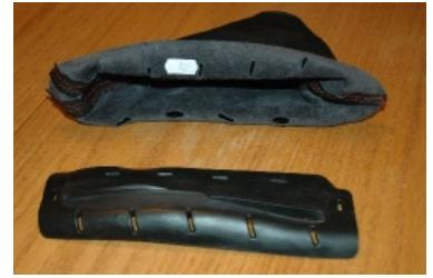
**8.** Next, position the new RedlineGoods boot in position and with a pen, mark the positions you need to cut slots in the leather for the retaining tabs. Play around with the boot to make sure it looks the way you want it to before you cut the slots. I used a pair of wire cutters to make the slots. I made them about 1/16th of an inch wide to facilitate slipping the boot over the retainers.
