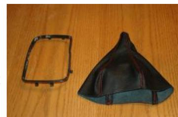
4. Remove the factory boot from the ring and replace with the RedlineGoods shift boot.
