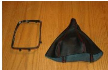
**4.** Remove the factory boot from the ring and replace with the RedlineGoods shift boot.
