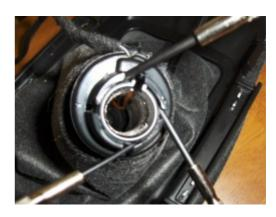
**11.** Remove the staples from the bottom side by straightening them out and pulling up from the top.
