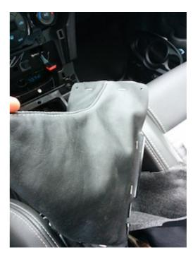
**17.** Guide the black piece onto the shift stick and slide the reverse lockout assembly back onto the stick so that the top of the stick protrudes through the silver piece.
