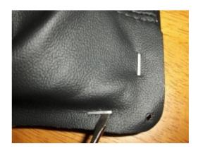
**15.** You can install the new boot onto the frame by lining the frame with super glue or by stapling the boot to the frame using the factory staple locations. I used small spring clips to hold the boot in place while stapling the boot on the frame.
