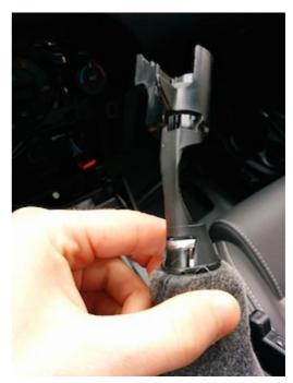
**8.** Use two flathead screwdrivers to hold open each of the two black clips on the reverse lockout. Then, pull the silver piece free of the black piece to separate the two pieces.
