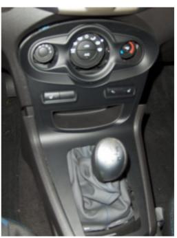
**29.** Push the cover back into the clips, starting with the upper portion at the heater controls, then moving to the lower portion over the boot.
