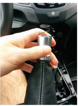
**13.**Remove the staples from the base frame attached to the old shift boot by straightening them out and pulling them from the top using needle nose pliers like this:
