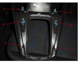
**4.** The connectors will have to be removed before the cover can come all the way off.
