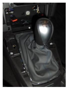
**28.** Set the console cover back on top of the console and reconnect any wires if needed.
