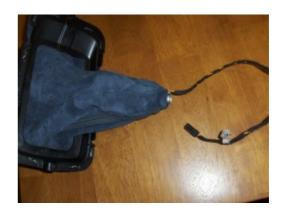
**23.** Retention ring installed on knob. There are 4 individual clicks that should be heard when the ring is pressed onto the knob.
