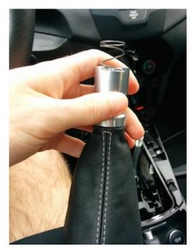
**12.** Push the two pieces together so that you hear and feel the silver piece clip back into the black piece. It may take some force to clip the pieces together but it will work. You can also carefully flip the boot inside out and push the clips inwards with a screwdriver until they clip.
