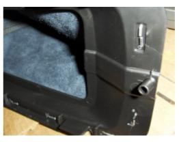
**21.** Boot inverted to install the shift knob.
