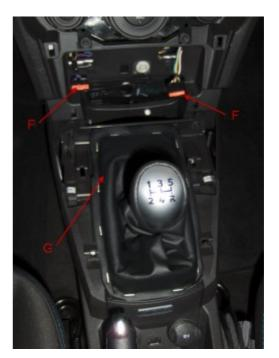
**6.** If you have an illuminated shifter you'll have to disconnect the power connector and unclip it from the shifter stick.
