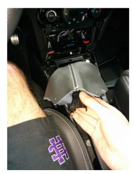
**10.** Slide the black piece up under the new shift boot, so that the top of the black piece sits flush with the top of the shift boot, as pictured. You can use a very small dot of super glue between the boot and the black piece in order to hold the boot and the black piece flush and properly aligned. Only use one very small dot so that the boot and black piece can be separated just in case of an error.
