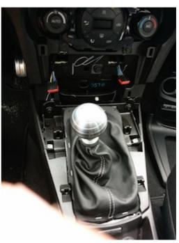
**19.** Push the frame down into place. There are notches to align it.
