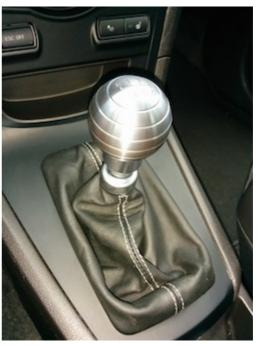
**21.** Push the cover back into the clips, starting with the upper portion at the heater controls, then moving to the lower portion over the boot.
