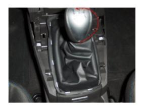
**8.** Once the boot and shift knob are off the stick, the lock ring has to be removed to release the boot from the knob. The arrows in the second picture below point to the 4 pieces of the lock ring that need to be released.
