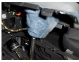
**26.** Screw knob back onto stick. This is easier to do with the boot bunched up towards the knob.
