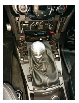
**20.** Set the console cover back on top of the console and reconnect the wires.
