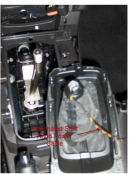
**7.** Unscrew the shift knob. The boot will have to be spinning with the knob, as well as the power cable for the illuminated knob if you have it.
