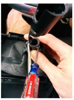
**9.** Hold the shift boot as if you were to install it, with the longer side of the base facing the front of the car. In order for the reverse lockout to work properly, you need to make sure that the black plastic part that extends down and to the left must be facing the drivers side of the car (as noted in Step 6). You will notice if you did this wrong once everything is reinstalled.
