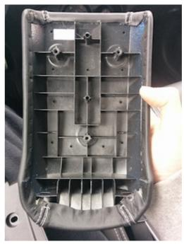
**4.** Place the wrapped armrest back on top of the armrest assembly, making sure it fits snug.
