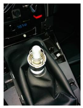
**18.** Screw the shift knob all the way back on to the stick. Make sure the reverse lockout still functions properly. Here you will be able to tell if you properly followed steps 9 and 11. If the reverse lockout is not working properly, revisit steps 9-11.
