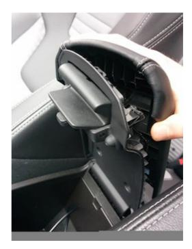
**3.** Glue or staple the new cover on the armrest. DO NOT remove the stock wrapping, put ours over it.
