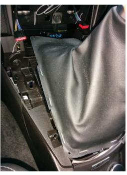
**7.** Flip the boot inside out so that the reverse lockout can be removed from the boot.
