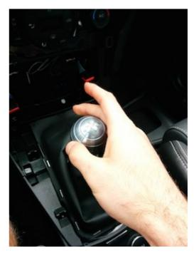
**6.** Lift the shift boot of the console with the reverse lockout still attached. Before doing so, take note of the position of the black piece and how it functions as a lockout. The part that extends down and to the left must be on the drivers side of the car when reinstalled on the new boot.
