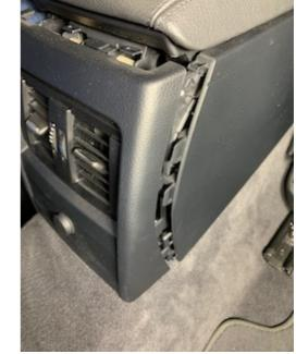
**16.** First use some sort of plastic pry tool like the one shown to separate the center console into two pieces as shown. Disconnect the lighter power and remove the console piece from vehicle.
