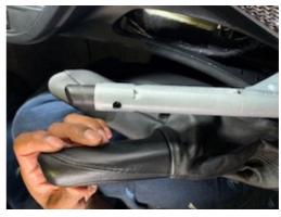
**13.** Flip the boot inside-out, slide it on the ebrake handle. Secure with tip-zie.
