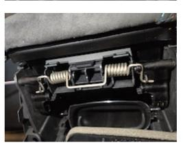
**24.** Now push silver pins into their slots and open the armrest as shown to make setting the spring easier.
