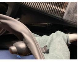
**12.** Pull firmly on handbrake handle until it comes off handbrake lever OR cut the zip-tie mounting the boot to the handle.
