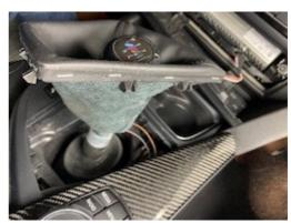
**3.** Disconnect this it is the cable to supply power for the lights on the shift knob.
