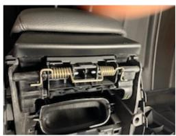
**19.** With the spring out of the way push on the silver pins as seen in the picture.
