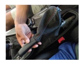
**14.** Work the boot down until the frame is again at the bottom, by the center console.
