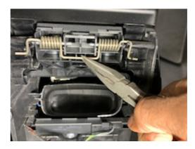
**18.** With the spring out of the way push on the silver pins as seen in the picture.
