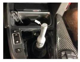
**9.** Push clips on shift boot into the area for the shift boot.
