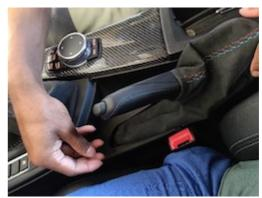
**15.** Push clips into place around the ebrake boot.
