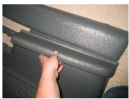
**7.** Install the RedlineGoods armrest cover - use contact cement to glue it over the stock armrest. Apply glue according to instructions on the glue can/bottle.
