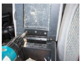
**2.** Remove the 9 small phillips head screws that are holding the black plastic cover on the armrest.
