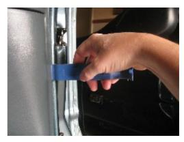
**6.** With door skin panel removed, remove 4 phillips screws which secure arm rest to door panel.
