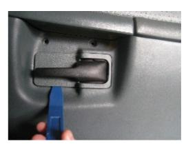
**4.** Remove interior door skin: Using a pry off tool, carefully start to remove door panel by prying off door retainer clips at all edges of door (except top-there are no retainer clips at the top).
