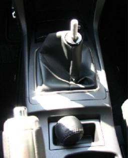
**3.** After you remove the first part of the center console you'll notice that it will still be attached by a wire clip. Unclip the wire and set aside the first part of the center console.
