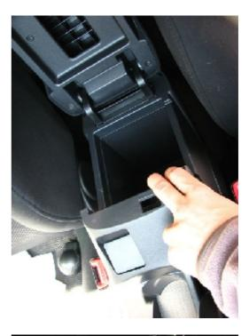
**4.** Next you will now see two screws holding the shift knob / ash tray / lighter assembly in place. Go ahead and remove these two screws with a Phillips screwdriver.
