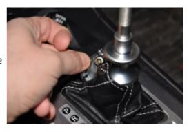
**3.** Open the arm rest and lift up the centre cup holder console from the rear, then slowly moving forward, pull upwards on the console near the shifter base. There are 4 clips here, ensure you don't loose the two white plastic ones near the shifter base.
