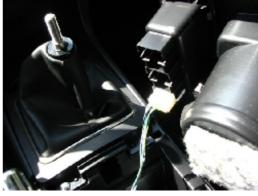
**5.** After you have removed the screws, gently lift up on the shift assembly. This should be a lot easier than the first piece you pulled out.
