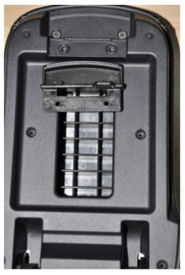
**16.** Remove two more screws under the plastic armrest lock clip and slowly remove the arm rest frame.
