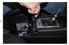
**7.** Unscrew the two screws holding the shifter base in place and set them aside.
