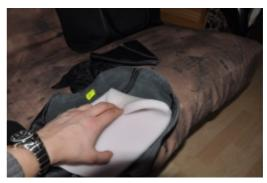
**20.** Once you have the Leather on the arm rest, stretch it out to your liking over the shell and clip in place with soft - pressure clamps.
