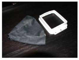
**12.** Next fit the new shift boot over the plastic shift boot frame assembly.
