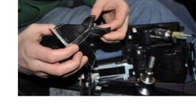
**11.** Remove the OEM shiftboot from the shift boot frame by pulling out the staples.
