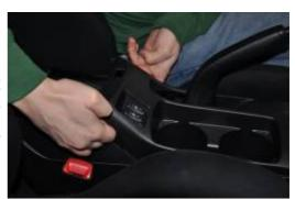
**3.** If you have a RalliArt or an EvoX MR, Unclip the AWC module wires by depressing the white tab. If you have a EvoX GSR simply set the cup holder trim aside as there is enough slack in the wire.
