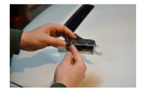
**12.** Place your new RedlineGoods shiftboot over the shifter boot frame ensuring the cutout goes to the bottom. Insert the shiftboot into the shift base console and re-tighten the three screws, then pull the shiftboot over the shifter stretching the elastic over the reverse lockout mechanism. Our shiftboot uses a durable elastic to strech over the reverse lockout instead of a button type clasp. This approach ensures a better fit and a cleaner looking end result.
