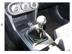
**2.** Open center arm rest console. Under it will be an area that you can pull on to take apart the first part of the center console. This will take a little of elbow grease to get it to pop off the first time. Be careful not to break any tabs along the way.
