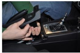
**6.** Unclip the heated seat module wires by depressing the white tab, and set the console aside.
