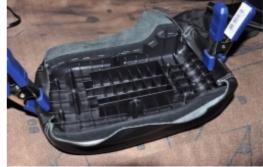
**21.** Staple the leather to the arm rest using 6mm - 1/4" or smaller staples. You may need to trim the leather around the corners like the OEM suede.
