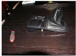
**8.** Next flip the shift knob / ash tray / lighter assembly over and unscrew the four screws and remove the shift boot assembly.
