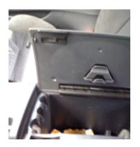
**10.** Install the arm rest cover, it comes with elastic so just slide it on and make sure it's aligned nicely (the decorative stitching should be even on the topside of the armrest). Then reverse step 9 to reinstall the armrest in the car.
