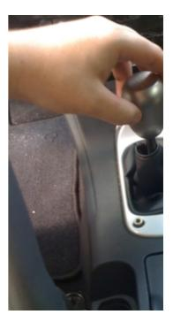
**5.** Loosen the top section of the center console by grasping the
