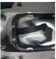
**7.** Remove the OEM boot from the bracket, and glue the new boot to it. Allow to dry. (The stronger the glue the better, you can use any epoxy-based glue to do the job, AutomotiveGOOP is one brand we've applied with good results, but there are many out there and you can get them at any RadioShack or similar store).
