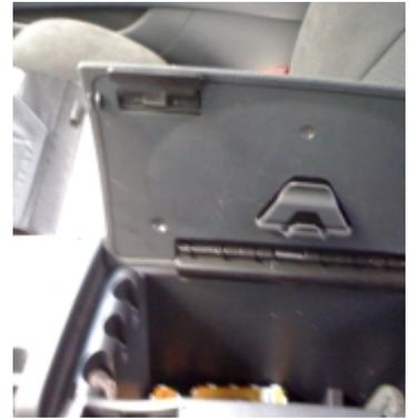
**10.** Install the arm rest cover, it comes with elastic so just slide it on and make sure it's aligned nicely (the decorative stitching should be even on the topside of the armrest). Then reverse step 9 to reinstall the armrest in the car.
