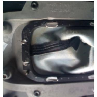
**7.** Remove the OEM boot from the bracket, and glue the new boot to it. Allow to dry. (The stronger the glue the better, you can use any epoxy-based glue to do the job, AutomotiveGOOP is one brand we've applied with good results, but there are many out there and you can get them at any RadioShack or similar store).
