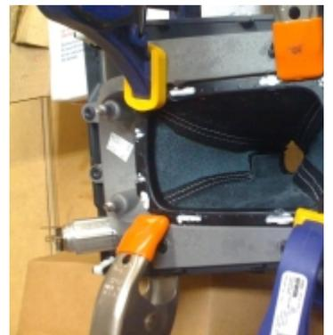
Now glue the bracket back to the console. You will need to put glue where the silver tabs were, use clamps to hold it down while it dries. Make sure you make it as secure as possible.
