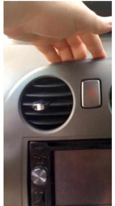
**3.** Remove the A/C controls unit, by grasping the top and bottom. No need to unplug it, because it can be replaced after step 5, it just needs to make room for the main console piece to come out.
