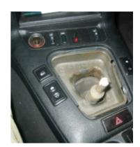
**3.** Now that the shift boot and its trim are out, carefully remove the vinyl boot from the frame (an x-acto knife will work great for that purpose). Clean the frame carefully with sandpaper of any glue/vinyl residue.
