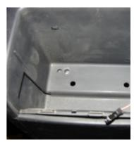
**3.** Use the philips scredriver to remove the spring, just dislodge it from the catches and it will come off easy.
