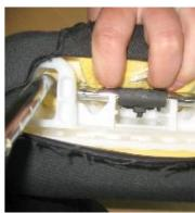
**11.** Your further steps are thus: removing the cover from the foam (which will now be very flexible and easy to work with since the rigid structure from within had been removed), installing the new cover on the foam and reinserting the structure into the foam now in the new cover.
