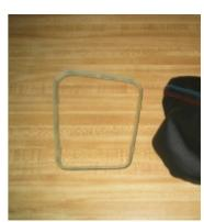
**4.** To install the shift boot you must glue the boot in the plastic frame. Any epoxy-based glue (3M makes some great glues for that purpose) will work perfectly. Just glue the boot in (make sure the shorter stitching is facing towards the front of the car).
