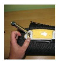
**10.** .Pull the stock headrest ALONG WITH THE FOAM off the structure. This will require moderate force.
