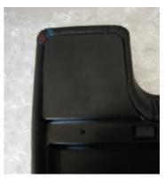
**10.** ... two screws near the hingest (hidden under little plastic circles you need to pry off)... and a bunch of latches. Wedge the inner trim with a flathead or small philips screwdriver to get it to disengage.
