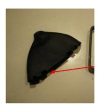
**6.** Once the leather and frame are attached, it is time to reassemble. Pop the Steptronic Faceplate back into place, and then pop the new boot into place.
