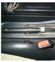
**7.** ... cut off the old boot, glue the new one and re-install.
