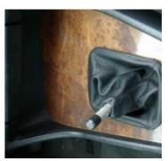
**7.** Press the shift knob back on to the shift rod until it snaps into place. You may have to turn it slightly to line up the slot in the top of the shaft with the knob.
