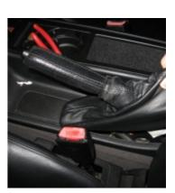
**8.** Pinch the boot and pull straight up. The boot is held in place by a snap-in plastic ring, which should come right out.
