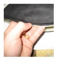
**17.** Allow the glue to dry; again, follow the directions supplied with your glue. When dry, pull the top of the boot down through the bottom, and slide it back over the brake handle.
