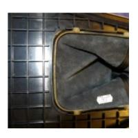
**6.** Slip the frame and boot over the shift rod and carefully press the frame down until it snaps in place. You may have to squeeze slightly in on the sides of the frame where the clips are to make it go down easier.
