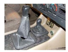
2. The base of the original boot is glued to a metal frame that is held to the plastic console by metal tabs. Fit a flat tool under the frame and carefully pop it up and off. Pull the old boot up and inside out, exposing the rubber O-ring that holds the boot onto the indentation on the hand-grip. Roll the O-ring down and off the grip. Remove the hand-grip from the shift stick by gripping it with both hands and turning it counter-clockwise.
