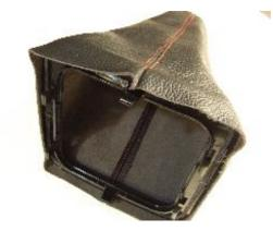
**5.** If necessary, use a sharp tool to cut the four corners of the new boot so it folds on the corners. Take care not to cut too long a cut.
