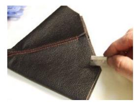
**6.** Use a good quality glue and apply glue to the frame. Fold the leather over the frame. Use clamps (clothes pegs) to hold the leather against the glued frame. Wait until dry.
