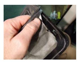
**4.** Place the frame inside the new boot, checking for fit and making sure to line up the stitching as desired.
