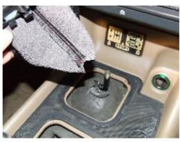
**9.** Using a hooked tool, pull the O-ring up and over the new boot so that the O-ring fits into the groove on the base of the hand-grip.
