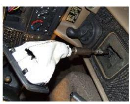
**3.** Pull the old boot and frame up and away. Pull the old boot off the frame. It is hot-glued. Take care not to twist the frame out of shape.
