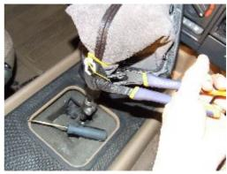
**11.** Pull the boot down and right-side-out. Fit the frame over the opening and push down securely. It may help to push the tabs carefully with a flat tool so they get past the plastic edge and "click in".
