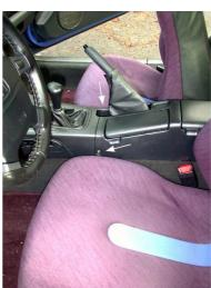
**3.** Remove the rear console section and slide it back (to completely remove it, you would need to unplug the cigarette lighter cable):
