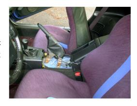
**4.** Unscrew the shift knob. It may be very tight, so if you cannot do it by hand, use vise-grips for extra leverage. Make sure to wrap the shift knob with a cloth or a towel to prevent from scratching it. Then remove the two screws holding the front section of the console:
