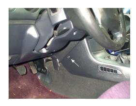
**5.** To completely remove the front section, gentle pry it rearward to free the two clips holding it to the upper dash above the stereo opening. Because it is blocked by the e-brake, you will need to lift the section upward while spreading the "wing" sides (where the screw holes are) and rotating it at the point of contact with the e-brake. After it's removed, turn over the front center console section for removal of the shift boot collar - there are two screws that hold it into place:
